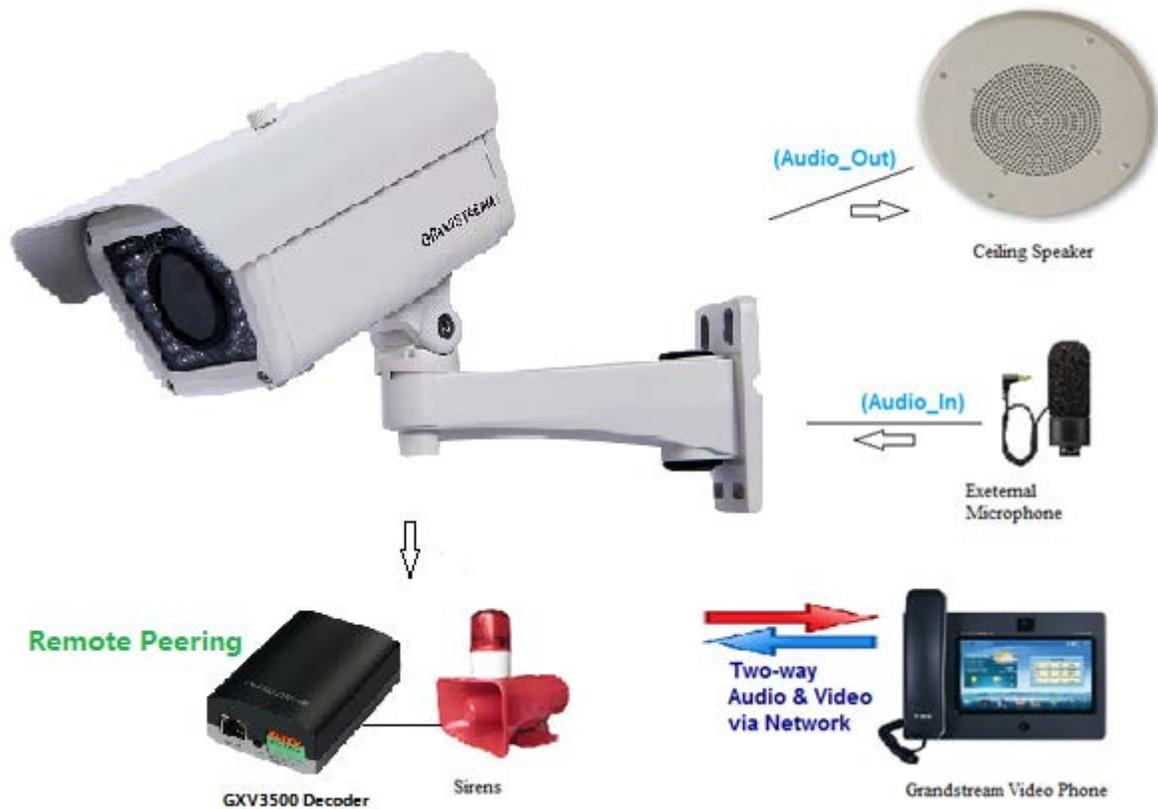
**Figure 6: Application Peripheral Connection for GXV3674\_HD/FHD\_VF v2**
