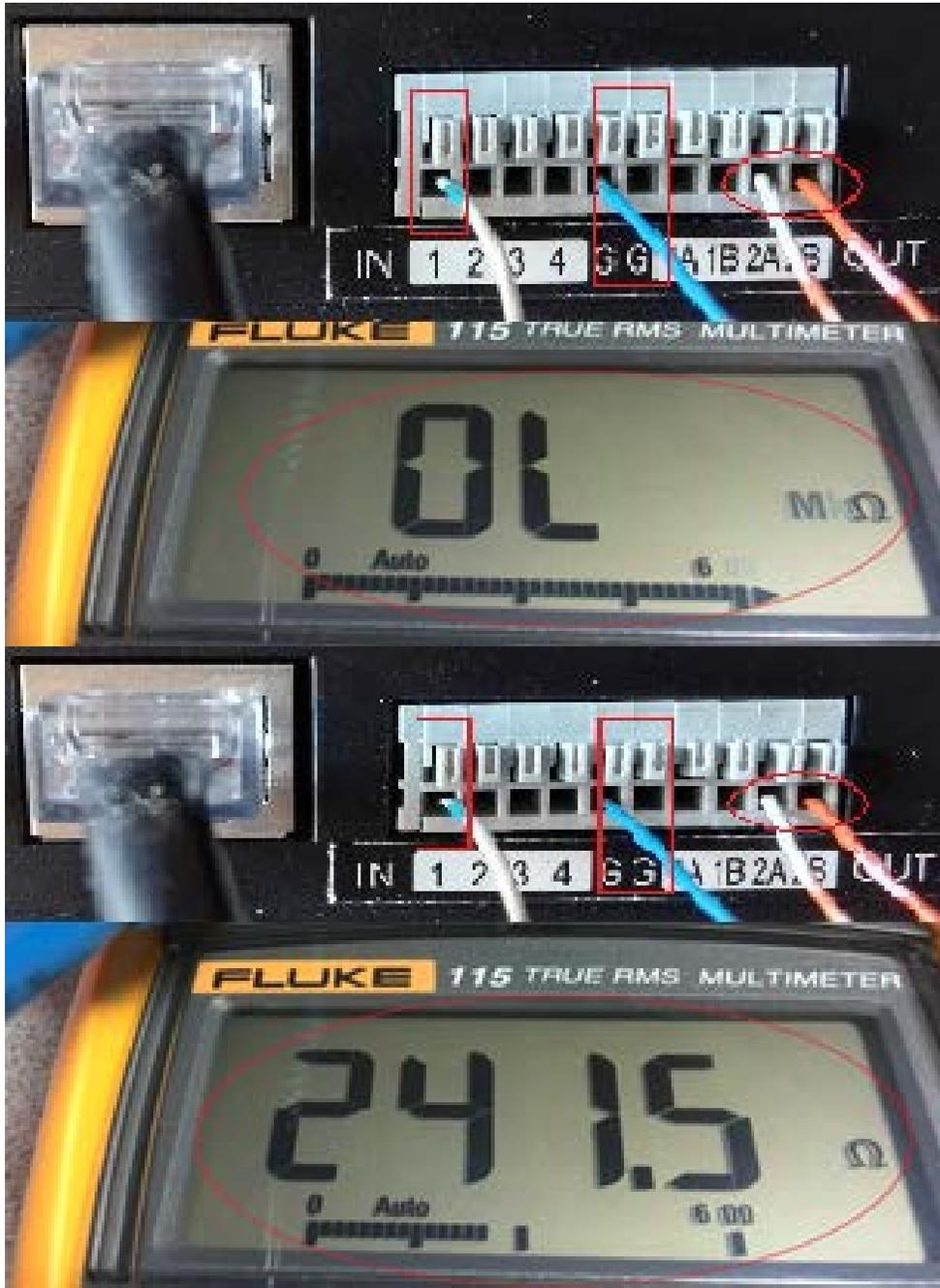
**Figure 25-4: GVR355X Alarm\_Out Circuit Measurement**
