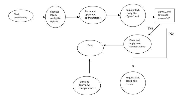
Figure 1: Provisioning Flow.
