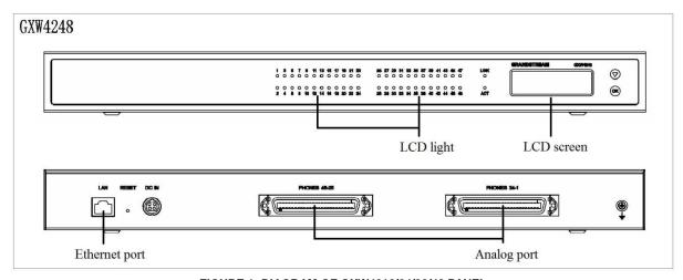
FIGURE 1: DIAGRAM OF GXW4216/24/32/48 PANEL
