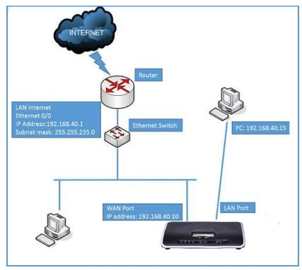
Figure 12: UCM6202 Network Interface Method: Switch
